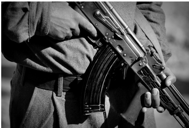
Figure 4.62 A Hungarian AMD-65 in the hands of a member of the Afghan National Police. Although it is an AK-pattern rifle, the AMD-65 is distinguishable by its forward vertical fore grip that is an exact copy of the pistol grip and by the selector-switch markings: The center position is the symbol for infinity, and the lowest position is the numeral 1. A semiautomatic version of the AMD-65 is manufactured as the SA2000M or SA65M, produced as such by Fegyver or using a U.S.-made receiver. (U.S. Air Force image; photographer Staff Sgt. Joseph Swafford.)
